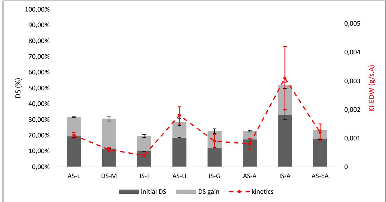
Figure 3: EDW tests performance for different sludges (final DS and dewatering kinetics)
