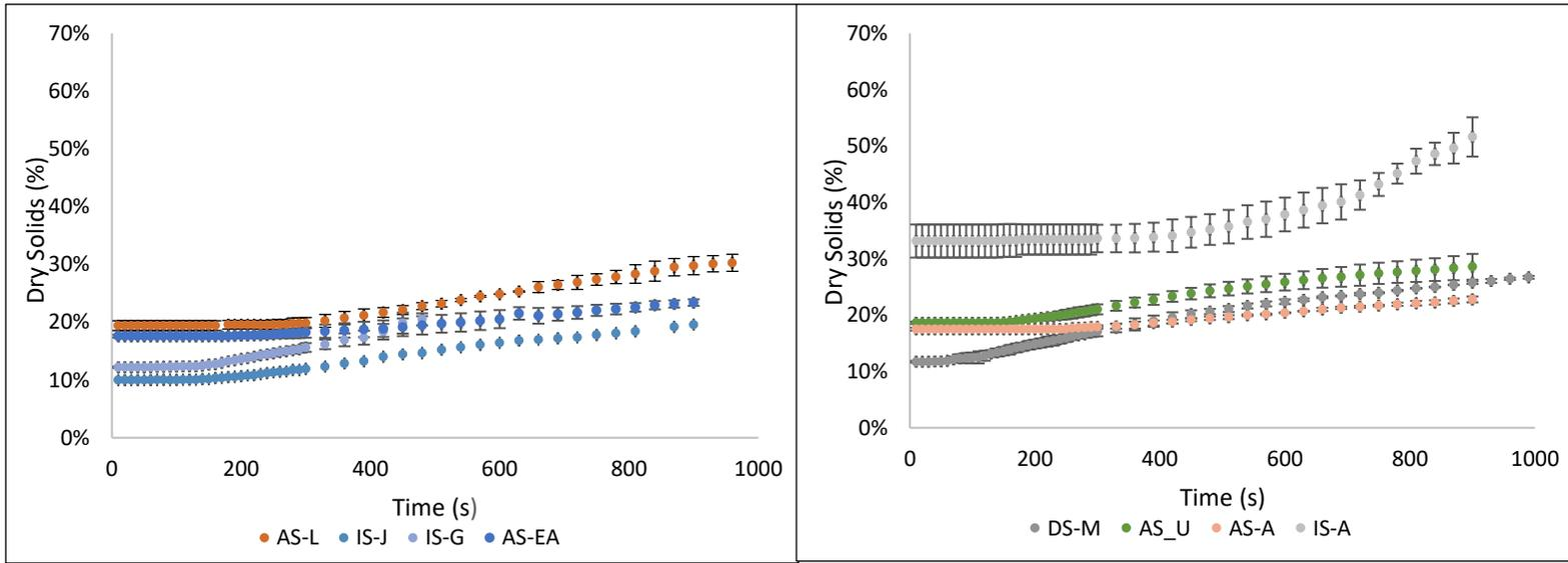
Figure 2: evolution of dry solids content over time during electrodeewatering tests
