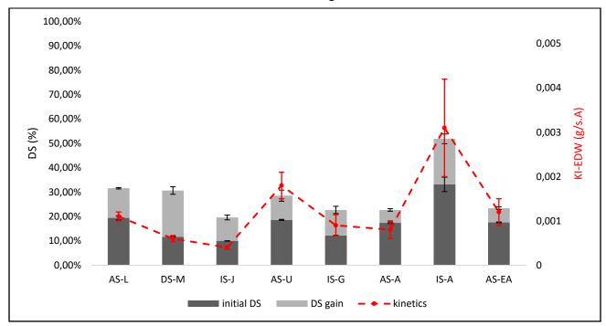
Figure 3 represents the results of evolution of DS content and the dewatering kinetics coefficient differences between all the tested sludges.
