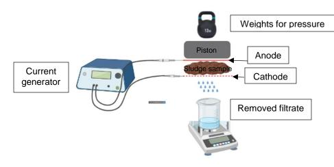
Figure 1: experimental setup
