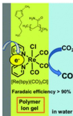
Figure 6. fac -[Re(bpy)(CO) 3 Cl] ([Re–Cl]) dispersed in polymer ion gel (PIG) ([Re]–PIG) to carry out electrocatalytic CO 2 reduction in water. 26
