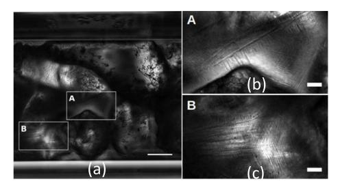
**Figure 12.** Feathered dendritic crystals of methane hydrate growing into capillary bridges between sand grains, at 7 MPa and -16 °C, in run 5: (a) Image with scale bar of 100 µm; (b) image corresponding to zone **A**, scale bar of 20 µm; (c) image corresponding to zone **B**, scale bar of 20 µm.
