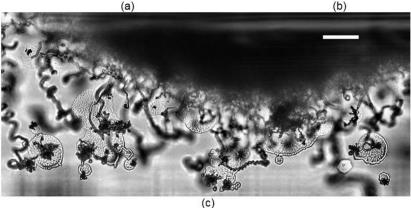
**Figure 4.** Methane hydrate filaments in run 5, growing into the gas from sand grains at 7 MPa and -16 °C. (**a**) A self-supporting filament; (**b**,**c**) Filaments drooping onto the floor of the glass cell, giving rise to localised halos. Scale bars: (**a**,**c**) 50 µm; (**b**) 20 µm.
