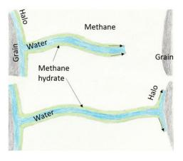
**Figure 14.** Proposed mechanism of the hydrate filament growth process (Figure 4). The filament is hollow and conveys water to its expanding tip (**top**), until its hits (**bottom**) the sand surface at the right and forms a halo radiating around the contact point.
