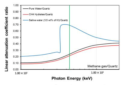
Figure 2. Linear attenuation coefficients relative to quartz vs. photon energy.
