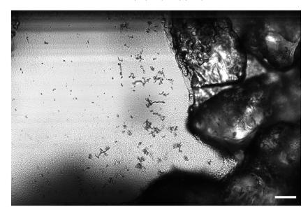
**Figure 5.** Methane hydrate halo and filaments on the floor of the glass cell on warming from -16 to -5 °C in run 5. Scale bar: 50 µm.
