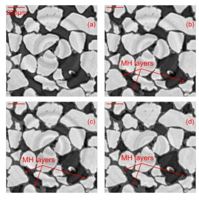
**Figure 9.** Tomographic sections of the thickening of methane hydrate (MH) layers in run 3 (**a**) 4 h following imposition of the MH formation conditions, (**b**) 10 h, (**c**) 15 h, and (**d**) 21 h.
