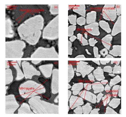
**Figure 8.** Tomographic sections of the growth of methane hydrate: (**a**,**b**) after 10 h following the imposition of formation conditions in run 2; (**c**,**d**) after 6 h in run 4.
