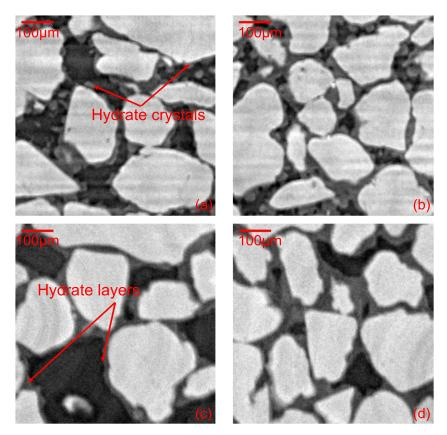
**Figure 10.** Methane hydrate morphologies: (**a**,**b**) images at two different locations within the sample in run 2, 18 h after the imposition of the MH formation conditions; (**c**,**d**) images at two different locations within the sample in run 3, 21 h after the imposition of the MH formation conditions.
