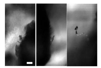
**Figure 7.** Examples of the shorter methane hydrate filaments growing from sand grains at 7 MPa, 2 °C in run 6. Scale bar: 20  $\mu$ m.
