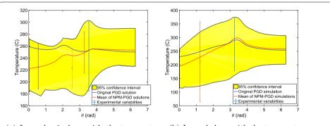
(a) Layer l-1 along with the temperature (b) Layer l along with the temperature measured by probes 1, 2, 3 and 4 illustrated sured by probes 1 and 2 illustrated in figure in figure 2(b) for set 2 of experimental pa- 2(a) for set 2 of experimental parameters rameters
