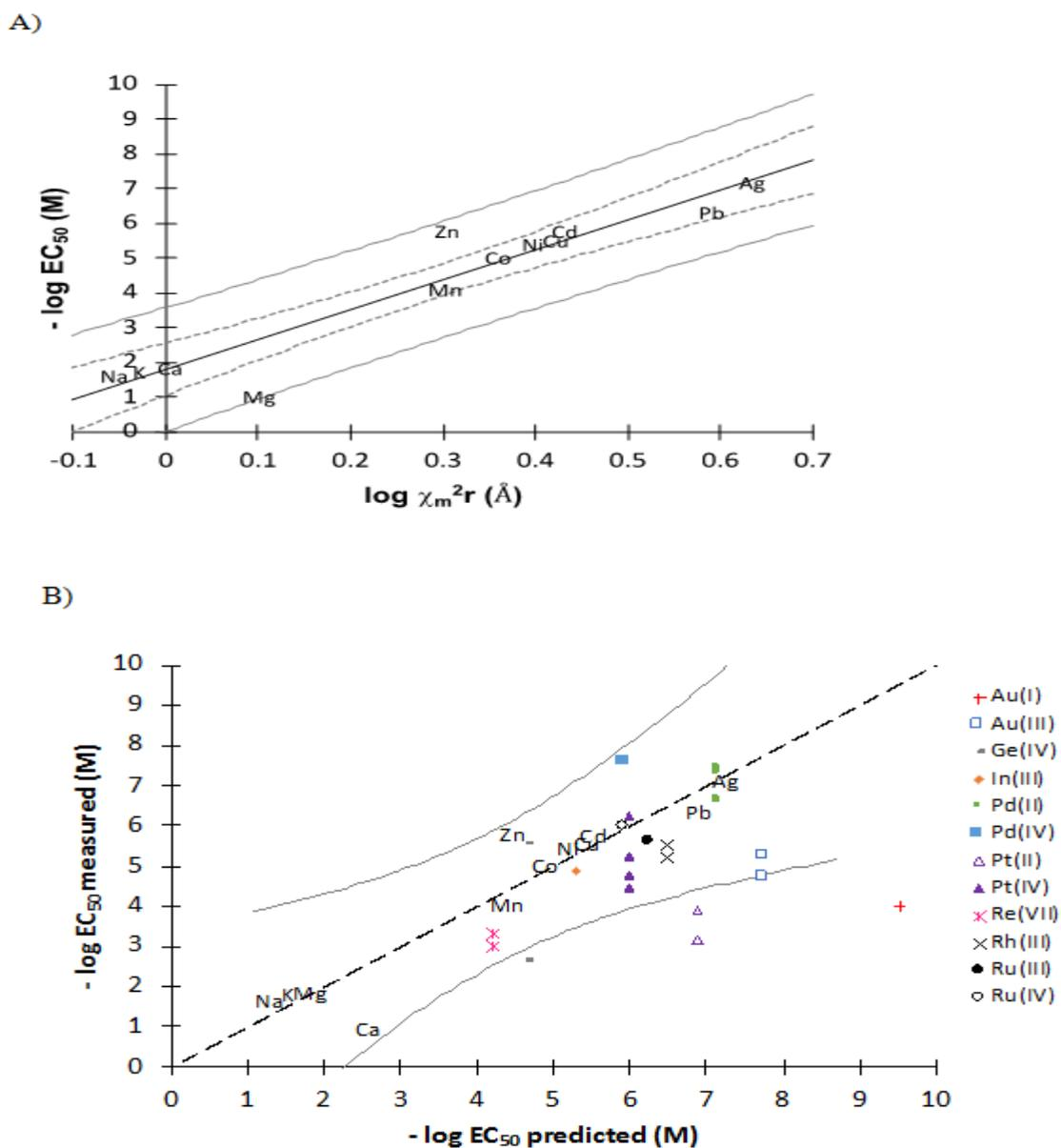
**Figure 2:** (A) Simple linear regression of the negative logarithm of the mean measured  $EC_{50}$  values of training metals (without algal species distinction), as a function of  $\log \chi_m^2 r$  ( $-\log EC_{50}$  predicted =  $1.816 + 8.607 \times \log \chi_m^2 r$ ;  $r^2_{adj} = 0.89$ ). The dotted and black lines represent the 95% confidence interval and prediction interval bands, respectively. (B) Linear regression between
