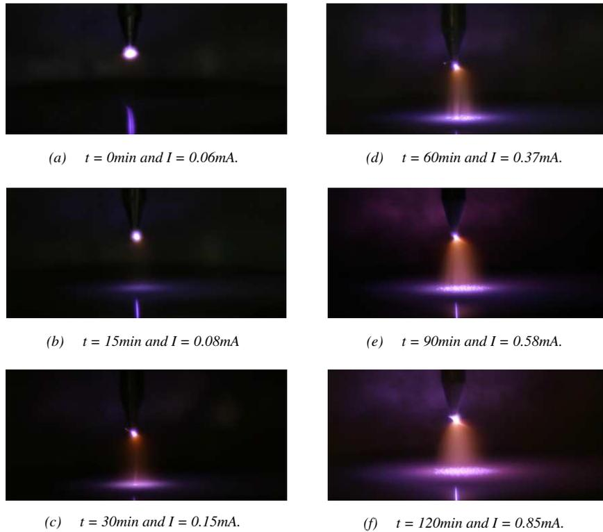
**Figure 5.** Photographs of optical phenomenon occurring between a single point and a plane during filtration activity.
