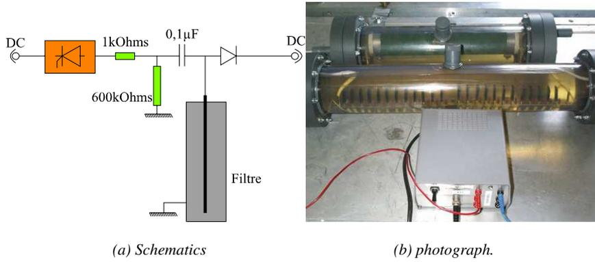
**Figure 2.** Hybrid pulsed power/direct voltage supply description.
