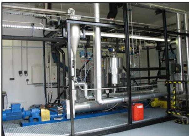
Figure 3—Photograph of the 165 bar hydrate loop.
