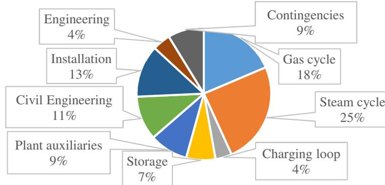
Fig. 2. Distribution of investment costs (102 M\$) for the base case: CCGT without combustion.
