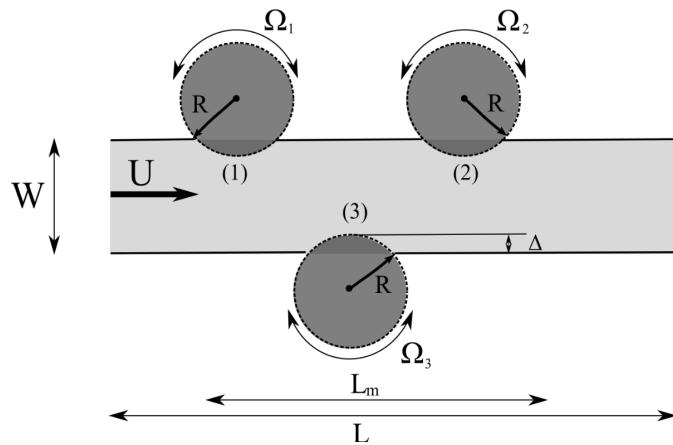
Figure 1 : Schematic illustration of the rotating arc-walls mixer.
