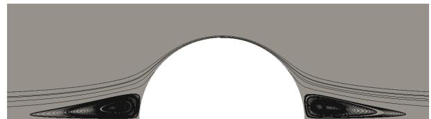
*Figure 1. Streamlines (Fraenkel solution on mesh e2: 40 000-Quad)*
