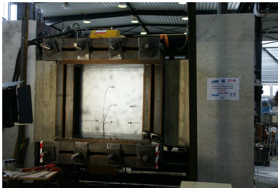
Figure 8 - DIC measurement system with the LVDT sensors
