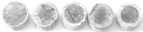
Fig. 4 – Mortar 1 degraded depth evolution with immersion time.
