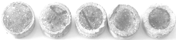
Fig. 4 – Mortar 1 degraded depth evolution with immersion time.
