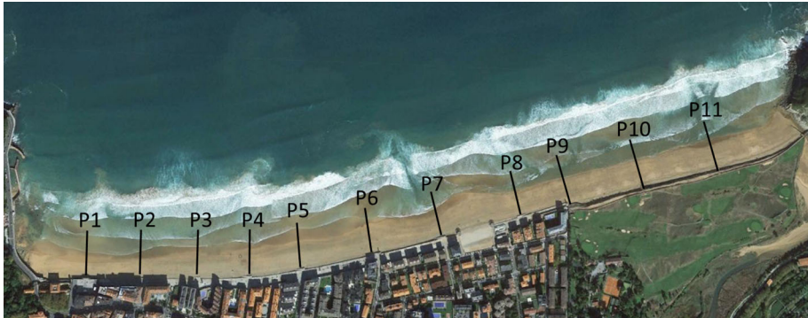
Fig. 3 Location of the eleven surveyed beach profiles used to calculate runup
